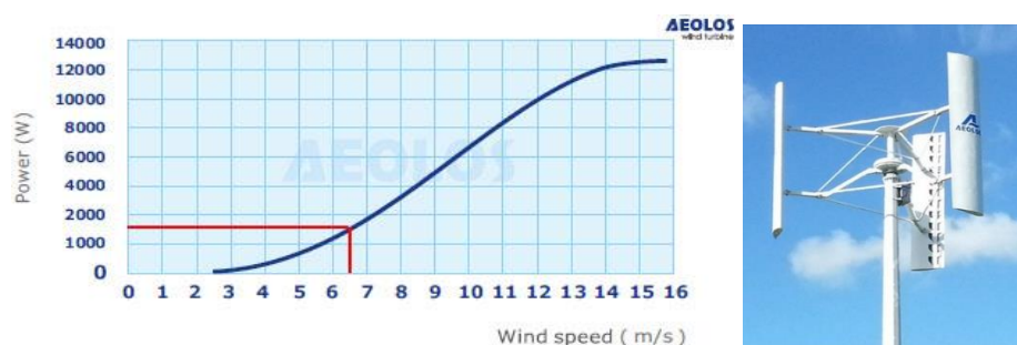
Figure 13. Power curves for 10 KW vertical Axis Wind Turbine [11].
